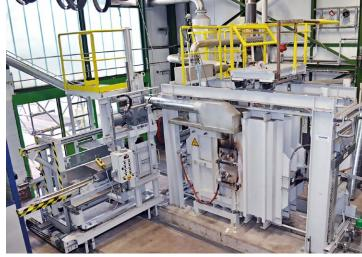
Expansion pressure generated by different coking coals is an important attribute which can cause damages of the coke oven wall refractory. Thus knowledge of the coking pressure of respective coal blend is an important variable for coke oven operation especially with reference to significant variability in the composition of coal charging blends.
